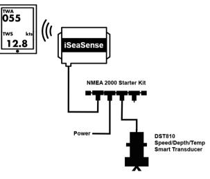
Basic cabling kit includes spare NMEA 2000 port and 1m connect cable for 3<sup>rd</sup> party display or device
