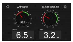
Analogue displays of wind information with true and apparent wind speed and angle available. Close hauled and speed trim displays too.
